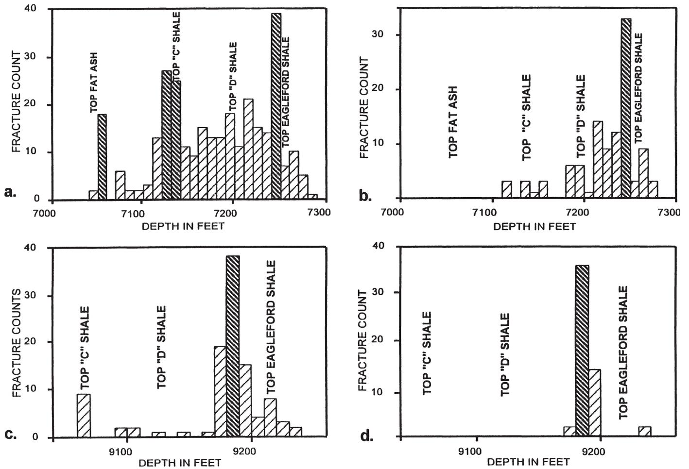
Figure 4. Fracture distributions in oriented cores from the Bell-Sample No. 1 and Robinson-Troell No. 1 wells: (a) Bell-Sample all fractures, (b) Bell-Sample oil-filled fractures, (c) Robinson-Troell all fractures, (d) Robinson-Troell oil-filled fractures.
